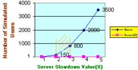
For example, if you have chosen a 2X-3X server capacity target, then this chart suggests that your WebSite server, as measured by the tests you have chosen, will saturate after the Nmax = 800 value shown. So, you have a server with a capacity of 800 simultaneous users.
