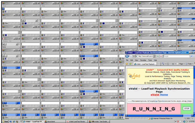
eValid LoadTest Running 100 Browser Users (BUs) on One Machine
